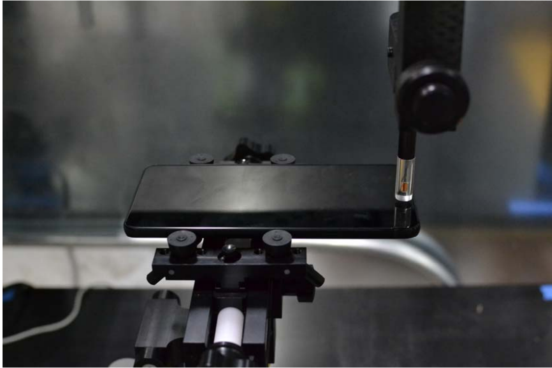
Figure 15-1 Test Setup for Wireless Device
