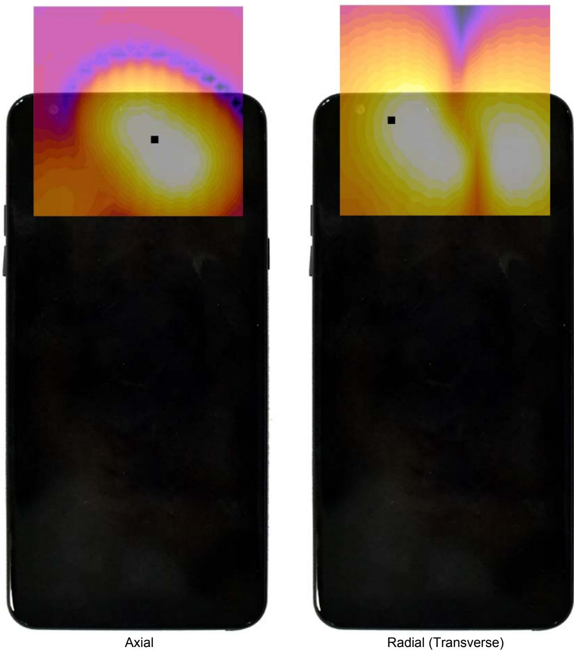
Figure 15-3 T-Coil Scan Overlay Magnetic Field Distributions
