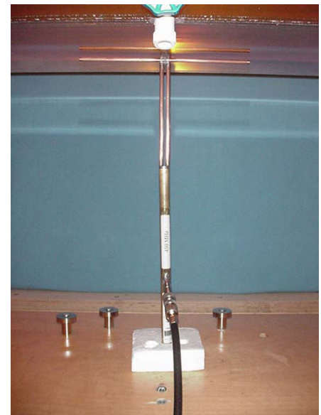
450MHz Dipole Setup
