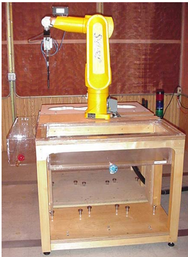
DASY4 SAR Measurement System with validation phantom
