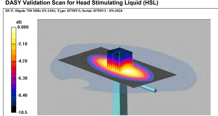
Communication System: CW 750; Frequency: 750 MHz; Duty Cycle: 1:1
