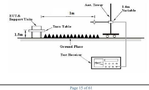
The radiated emission tests were performed in the 3 meters chamber test site, using the setup accordance with the ANSI C63.10-2013. The specification used was FCC 15.209, FCC 15.407 limits.
