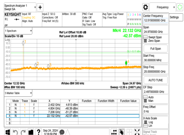
Spurious Emission_BLE 500k_LowCH00-2402MHz
