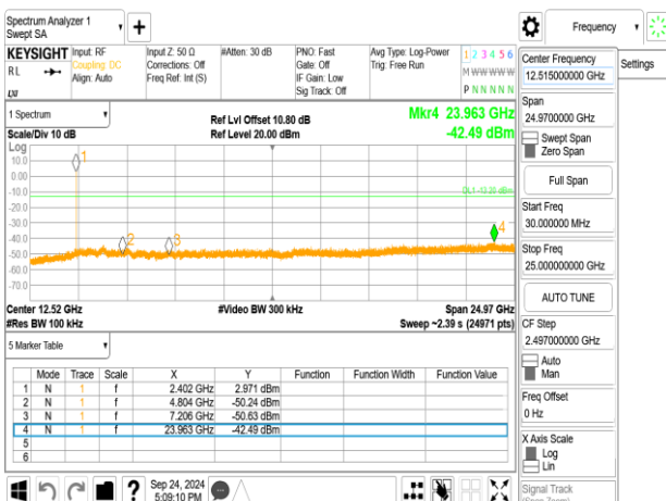
Spurious Emission_BLE 125k_LowCH00-2402MHz
