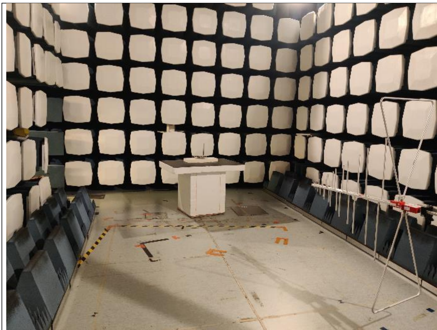
Picture 8, Radiated Emissions, common setup, 30 - 1000 MHz
