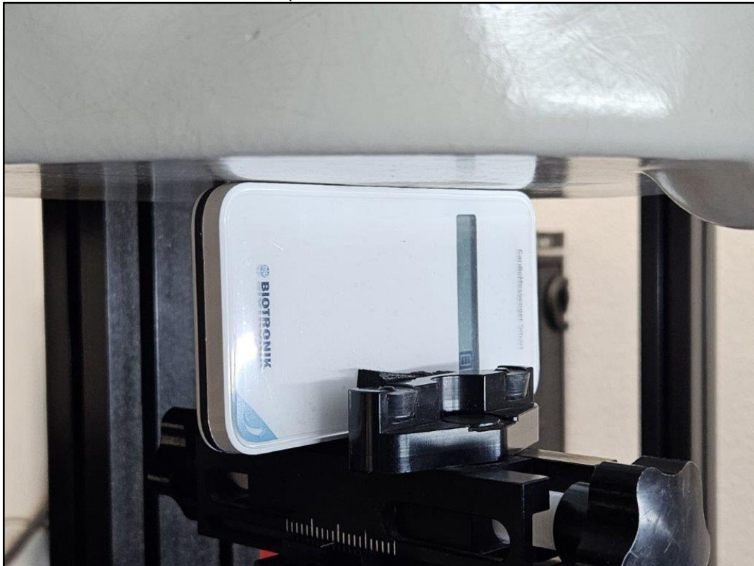
Photo 9: Test position left side with 0 mm distance
