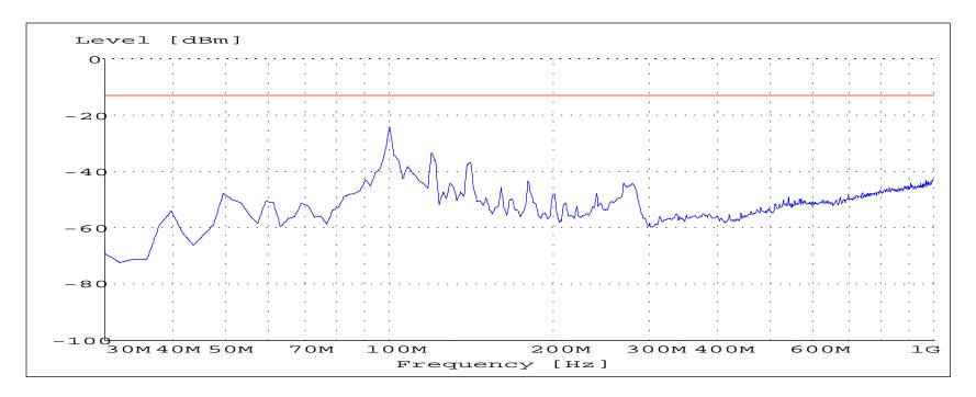
The emissions for all the channels were identical or a little bit lower. This is valid for both Transmit and idle mode.
