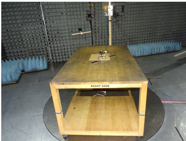
Photo 1: Test setup for radiated measurements
