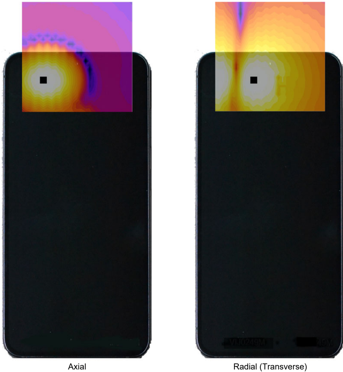
Figure 17-3 T-Coil Scan Overlay Magnetic Field Distributions
