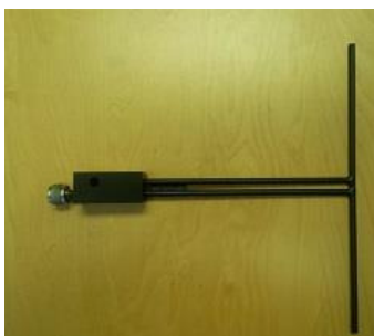
Figure 1 – MVG COMOSAR Validation Dipole
