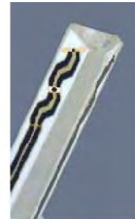
Figure E.2.2 Probe Thick-Film Technique
