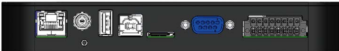
Figure 8 – Power, RS-232, USB, SDCard and LAN Connections
