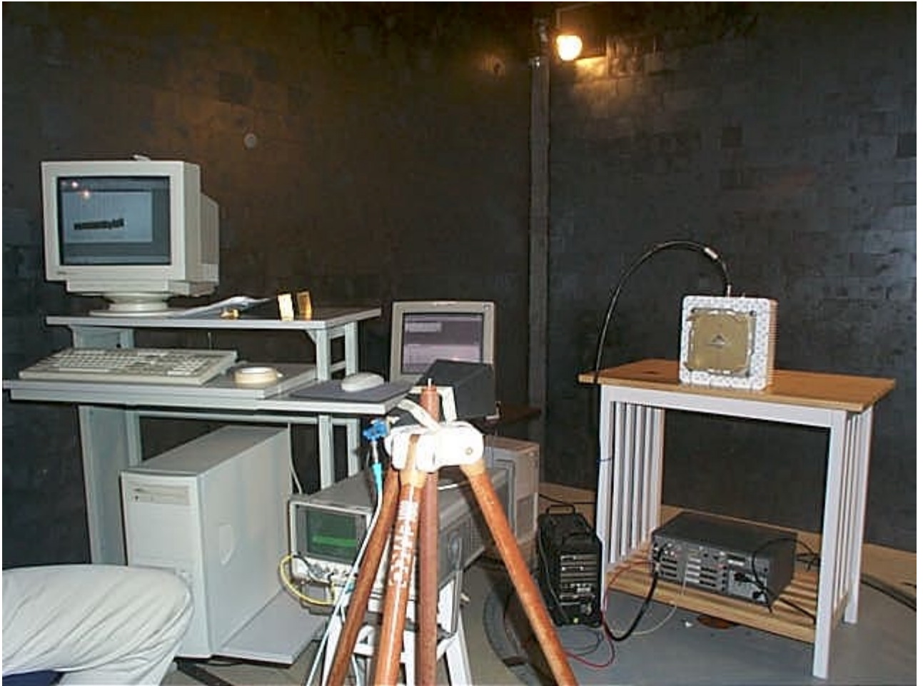
Figure 2 Radiated Spurious Emissions – Test setup
