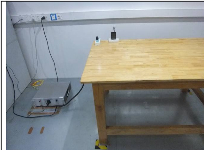
Conducted Emissions Test Setup Front View
