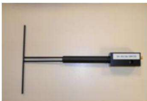
Figure 1 – Satimo COMOSAR Validation Dipole
