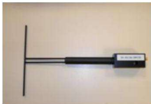
Figure 1 – Satimo COMOSAR Validation Dipole
