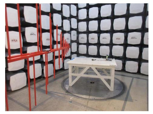
1.2 Radiated Spurious Emissions measured at 3 meters, 30 MHz to 1000 MHz, Rear View
