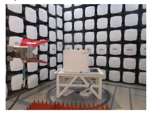
1.6 Radiated Spurious Emissions measured at 3 meter, 1 GHz to 18 GHz, Rear View
