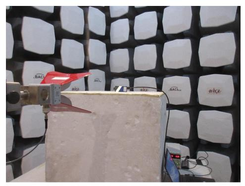
1.4 Radiated Spurious Emissions measured at 1 meter, 1 GHz to 18 GHz, Rear View
