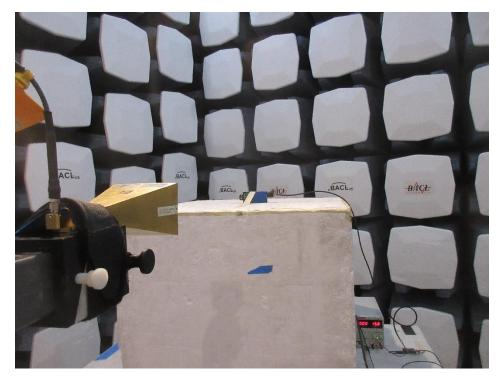
1.8 Radiated Spurious Emissions measured at 1 meter, 18 GHz to 26.5 GHz, Rear View
