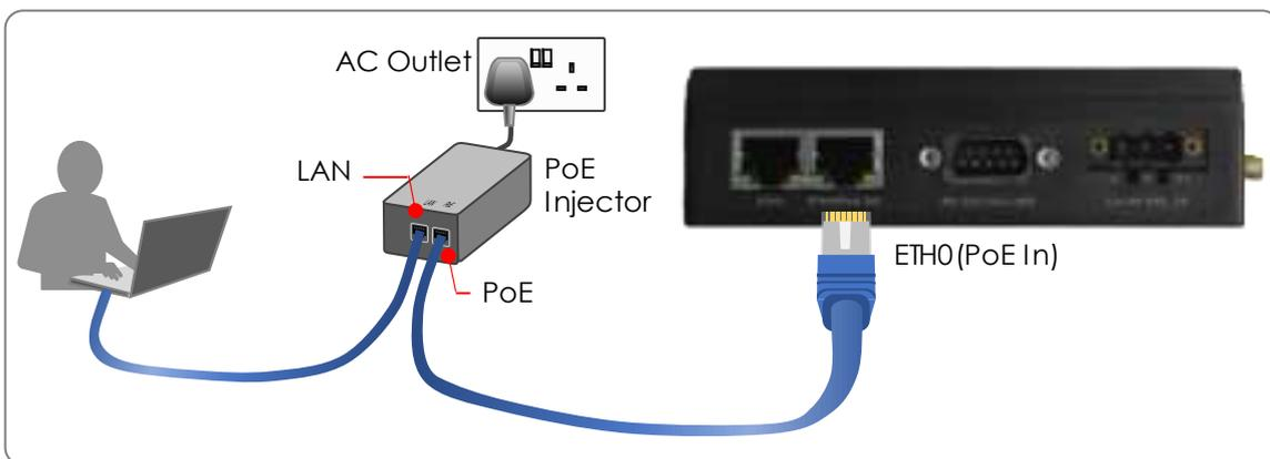
1. Connect the PoE injector's ports as follows with Ethernet cables.
