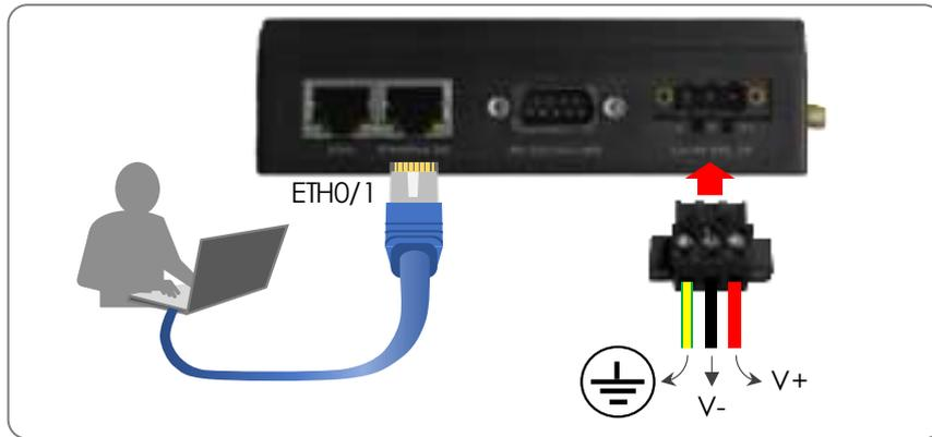
1. Insert ground/DC positive/DC negative wires (recommended AWG range: 12 – 24) into the terminal block. Use a small flat-blade screwdriver to tighten the wire-clamp screws so as to prevent the wires from loosening.
