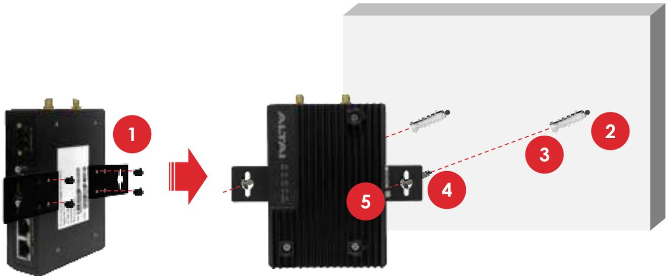
1. Drive the short screws to attach the two wall mounting plates to the unit.
