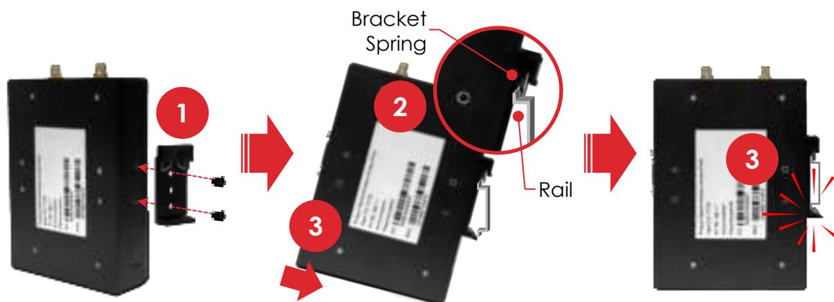
1. Drive the short screws (2 pcs) to attach the DIN-rail mounting bracket to the M360-X unit.
