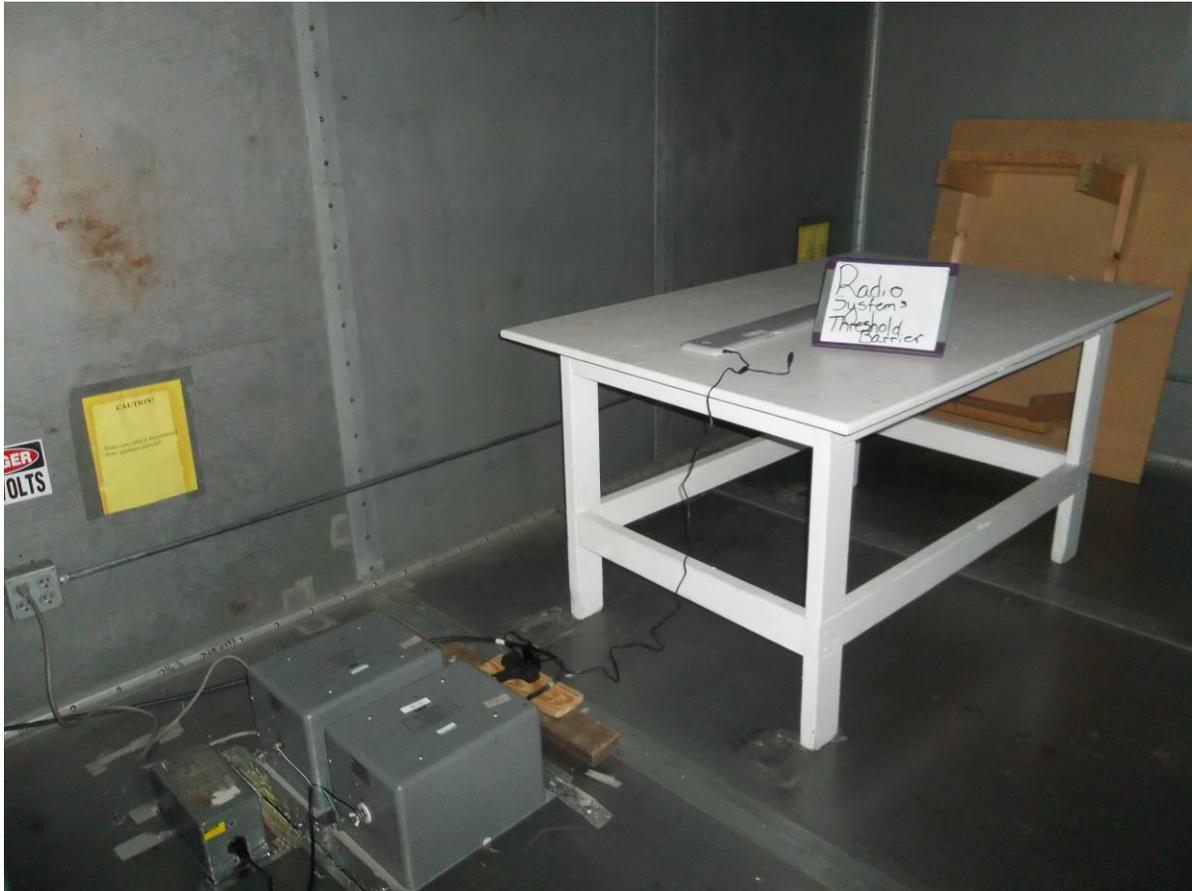
**Figure 5. Conducted Emissions Test Setup**
