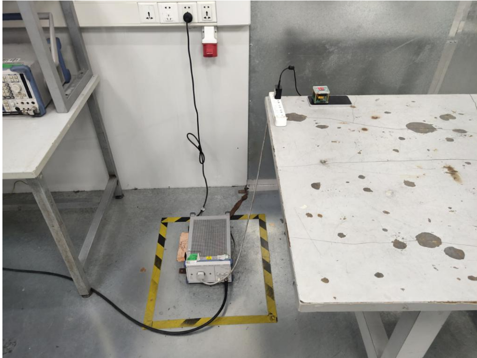
Photo of Conducted Emission Measurement
