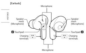
\*Make sure that the charging terminal is not soiled with foreign substance.
