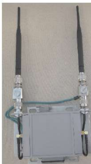
Figure 80 - Outdoor accessory kit mounting
