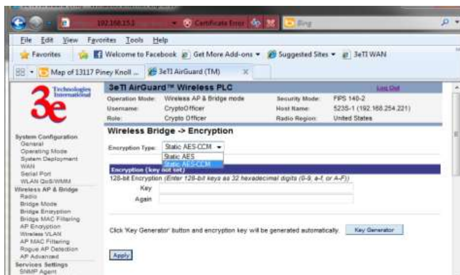
Figure 23 - . Wireless Bridge – AES-CCM Encryption
