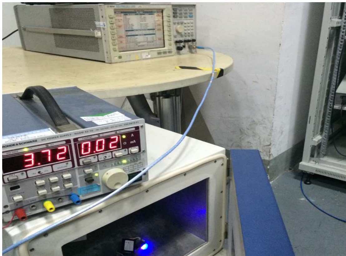
Frequency Stability Under Temperature & Voltage Variations Setup
