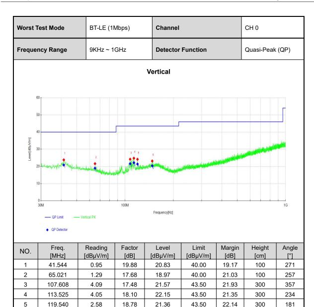
20.46 Remark: 1. 9kHz~30MHz have been test and test data more than 20dB margin.
