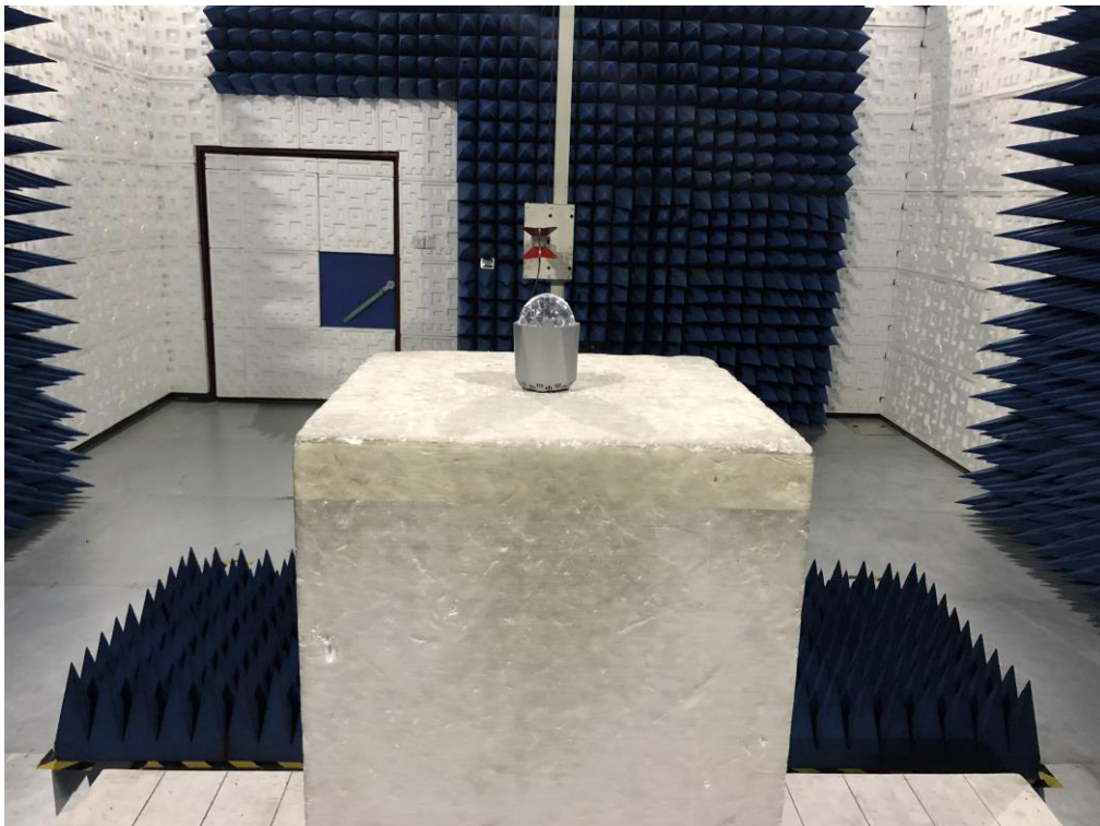
RADIATED EMISSION TEST SETUP ABOVE 1GHZ
