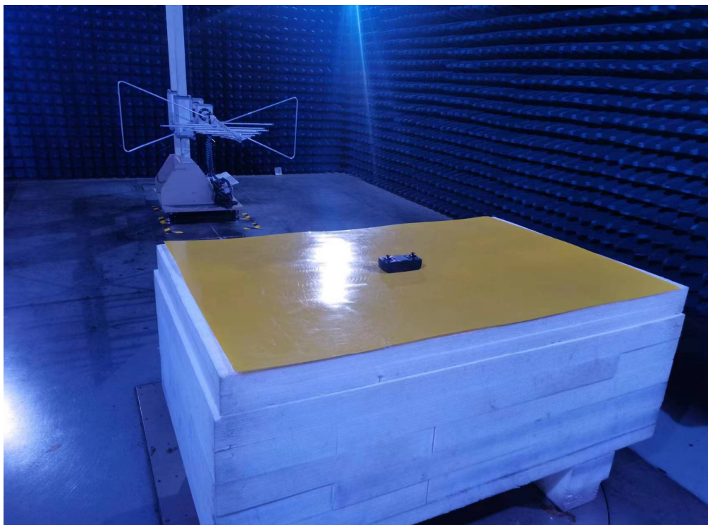
Photo of Radiated Emission Measurement (Above 1G)
