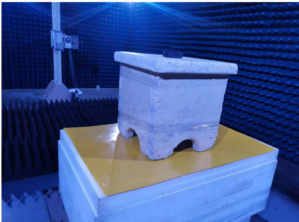
Photo of Radiated Emission Measurement (Above 1G)
