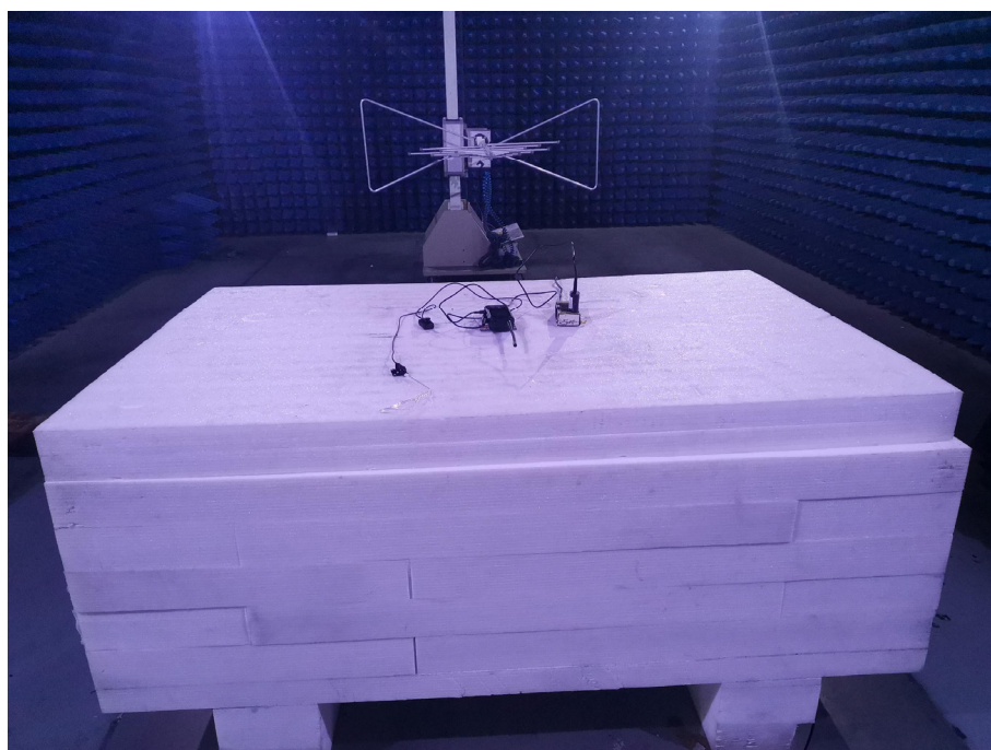
Photo of Radiated Emission Measurement (30MHz-1GHz)
