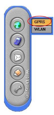
When users choose network configuration, the submenu will pop up. Left click the mouse on the GPRS item and the GPRS control panel will pop up. The current profile name and status of the GPRS configuration is displayed in this screen.
