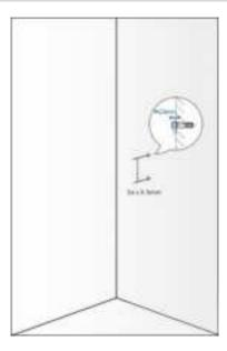
(2) Fix the mounting plate to the wall (pay attention to the orientation of the mounting plate). After adjusting the installation position, use two Philips pan head screws to secure the mounting plate to the wall.
