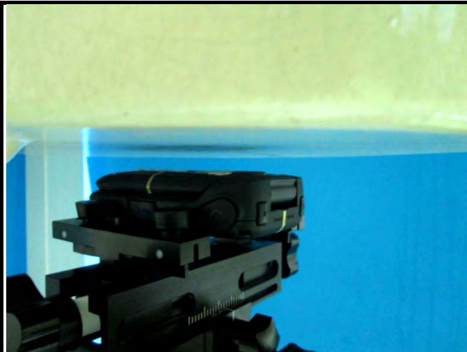
Front Face of EUT with 1.0 cm Gap
