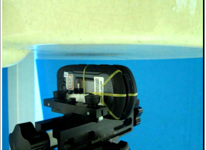
Right Side of EUT with 1.0 cm Gap
