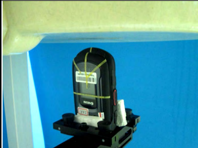
Bottom Side of EUT with 1.0 cm Gap
