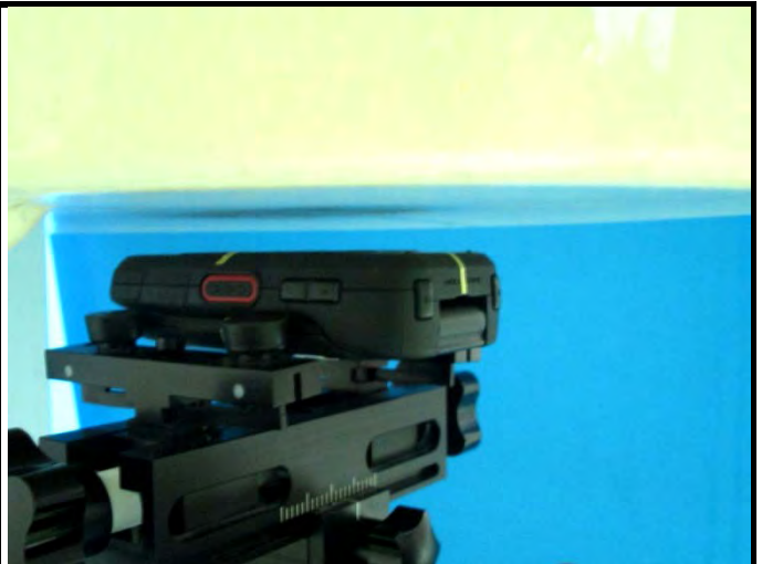
Rear Face of EUT with 1.0 cm Gap
