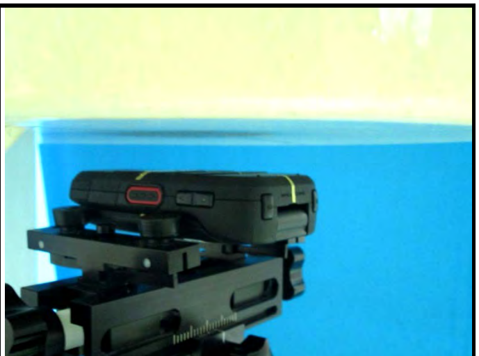
Rear Face of EUT with 1.5 cm Gap
