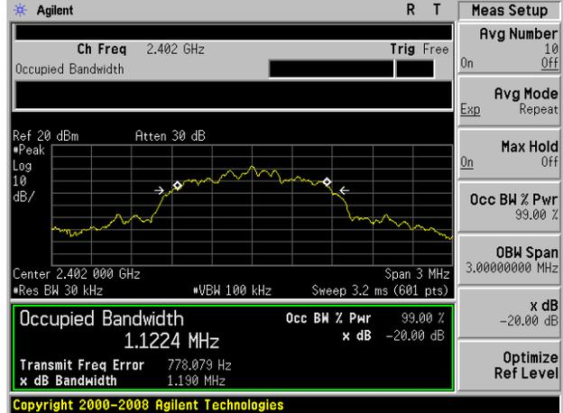
20dB Bandwidth plot on channel 39 (1Mbps)
