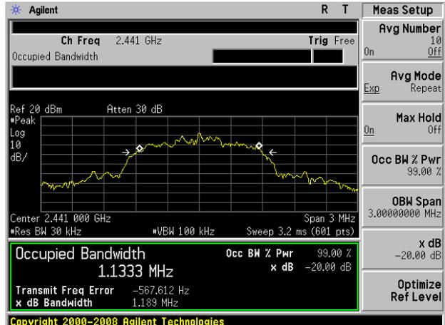
20dB Bandwidth plot on channel 78 (1Mbps)
