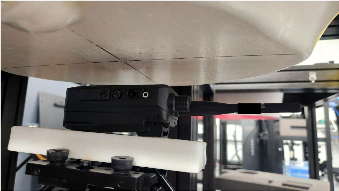
Figure C SAR Test Setup – Face – Front 25mm, Battery BP-315
