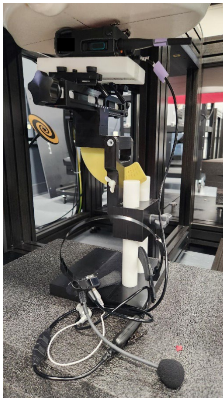
Figure I SAR Test Setup – Body– Back 0mm Default Battery BP-314 with Leather Case, Audio Accessory HS-102
