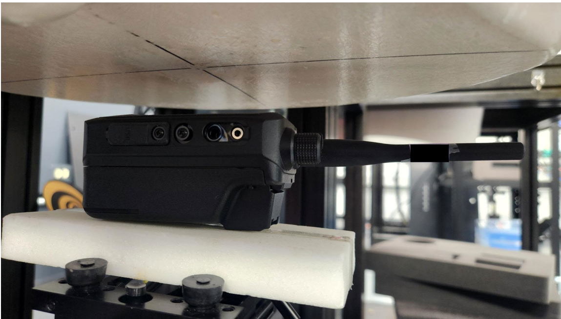
Figure B SAR Test Setup – Face – Front 25mm, Battery BP-291
