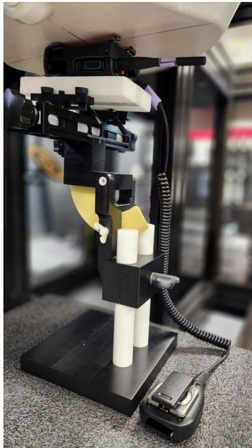
Figure D SAR Test Setup – Body– Back 0mm Default Battery BP-314 with Leather Case, Audio Accessory HM-222HLS
