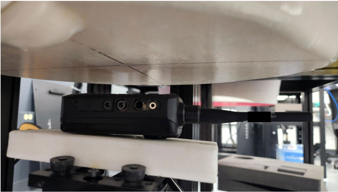
Figure A SAR Test Setup – Face – Front 25mm, Default Battery BP-314
