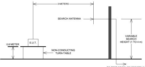
TO TEST RECEIVER/SPECTRUM ANALYZER EQUIPMENT: eLink Tag Tester FCC ID: HE7TTG
