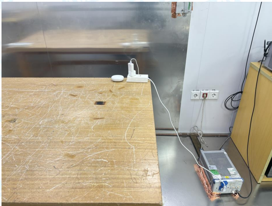
Photo of Setup for Conducted Emission
