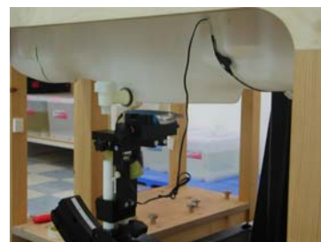
Fig. 19. Body SAR Test Setup with Holster
