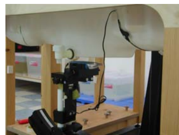
Fig. 18. Body SAR Test Setup with Holster
