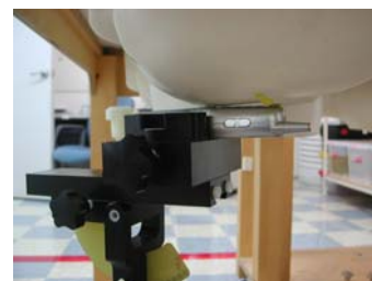
Fig. 16. Head SAR Test Setup
