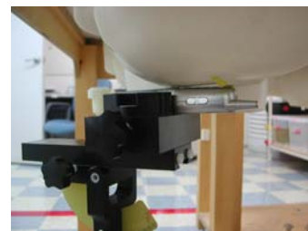
Fig. 17. Head SAR Test Setup
