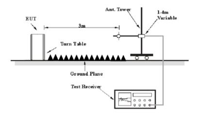
The radiated emissions were performed in the 3 meters distance, using the setup accordance with the ANSI C63.10-2013. The specification used was the FCC 15.209, and FCC 15.247 limits.
