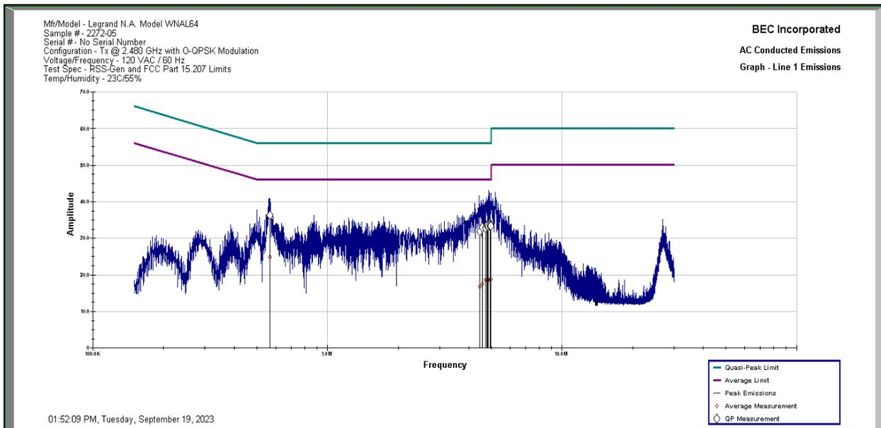
**Results:** All conducted emissions measured on the AC Power Port of the Legrand Model WNAL64 Sample 2272-05 in Tx Mode High Channel at 2.480 GHz are below the limit specified by FCC Part 15.207 and RSS-Gen 7.2 Limits by a margin of 19.81 dB.
