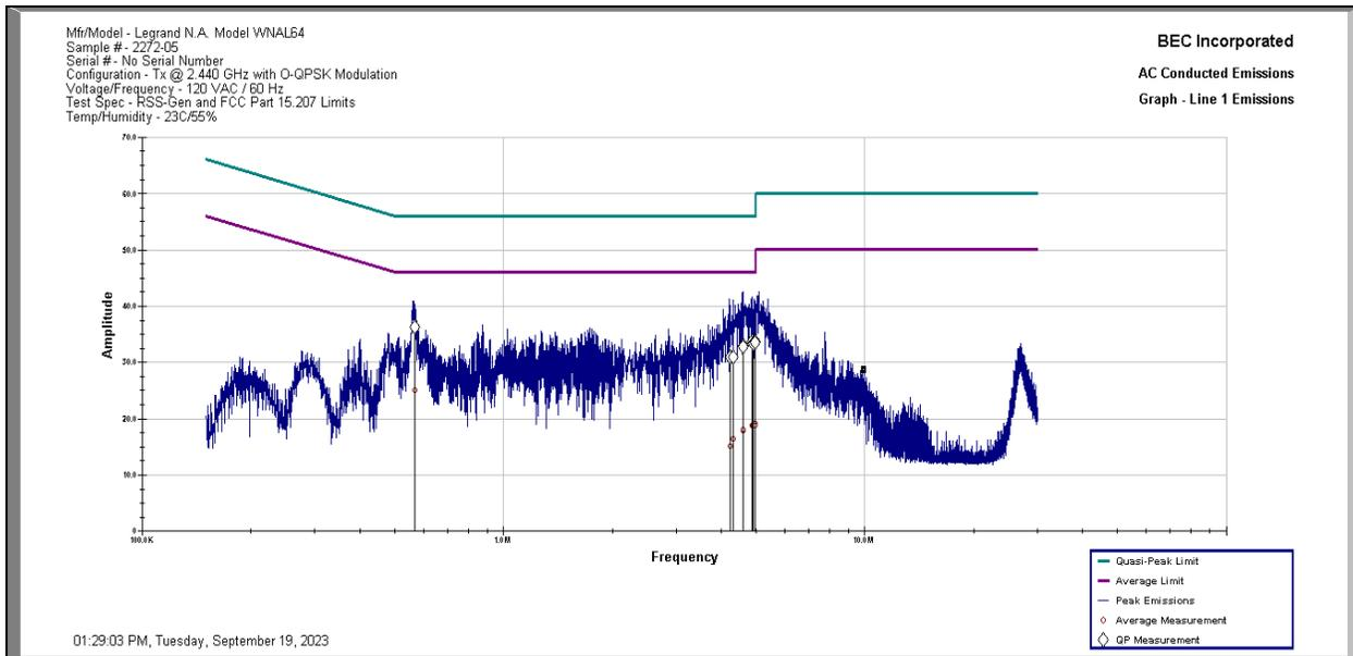
**Results:** All conducted emissions measured on the AC Power Port of the Legrand Model WNAL64 Sample 2272-05 in Tx Mode Middle Channel at 2.440 GHz are below the limit specified by FCC Part 15.207 and RSS-Gen 7.2 Limits by a margin of 19.67 dB.
