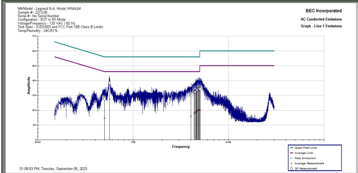
**Results:** All conducted emissions measured on the AC Power Port of the Legrand Model WNAL64 Sample 2272-05 in Rx Mode are below the limit specified by FCC Part 15.207 and RSS-Gen 7.2 Limits by a margin of 13.19 dB.
