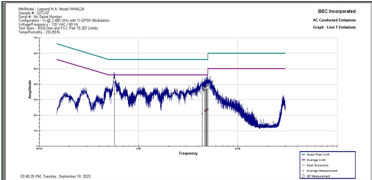
**Results:** All conducted emissions measured on the AC Power Port of the Legrand Model WNAL24 Sample 2272-07 in Tx Mode High Channel at 2.480 GHz are below the limit specified by FCC Part 15.207 and RSS-Gen 7.2 Limits by a margin of 12.2 dB.
