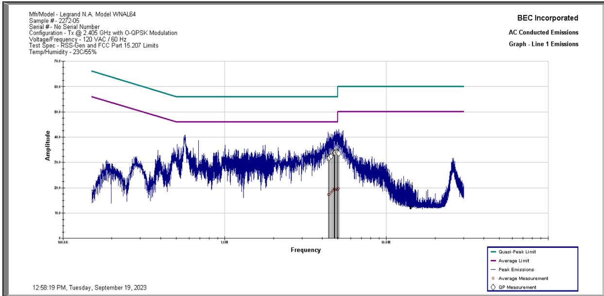
**Results:** All conducted emissions measured on the AC Power Port of the Legrand Model WNAL64 Sample 2272-05 in Tx Mode Low Channel at 2.405 GHz are below the limit specified by FCC Part 15.207 and RSS-Gen 7.2 Limits by a margin of 20.55 dB.
