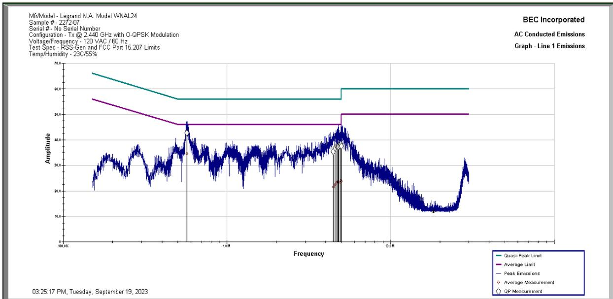
**Results:** All conducted emissions measured on the AC Power Port of the Legrand Model WNAL24 Sample 2272-07 in Tx Mode Middle Channel at 2.440 GHz are below the limit specified by FCC Part 15.207 and RSS-Gen 7.2 Limits by a margin of 11.38 dB.
