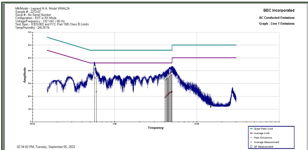
**Results:** All conducted emissions measured on the AC Power Port of the Legrand Model WNAL24 Sample 2272-07 in Rx Mode are below the limit specified by FCC Part 15.207 and RSS-Gen 7.2 Limits by a margin of 11.81 dB.
