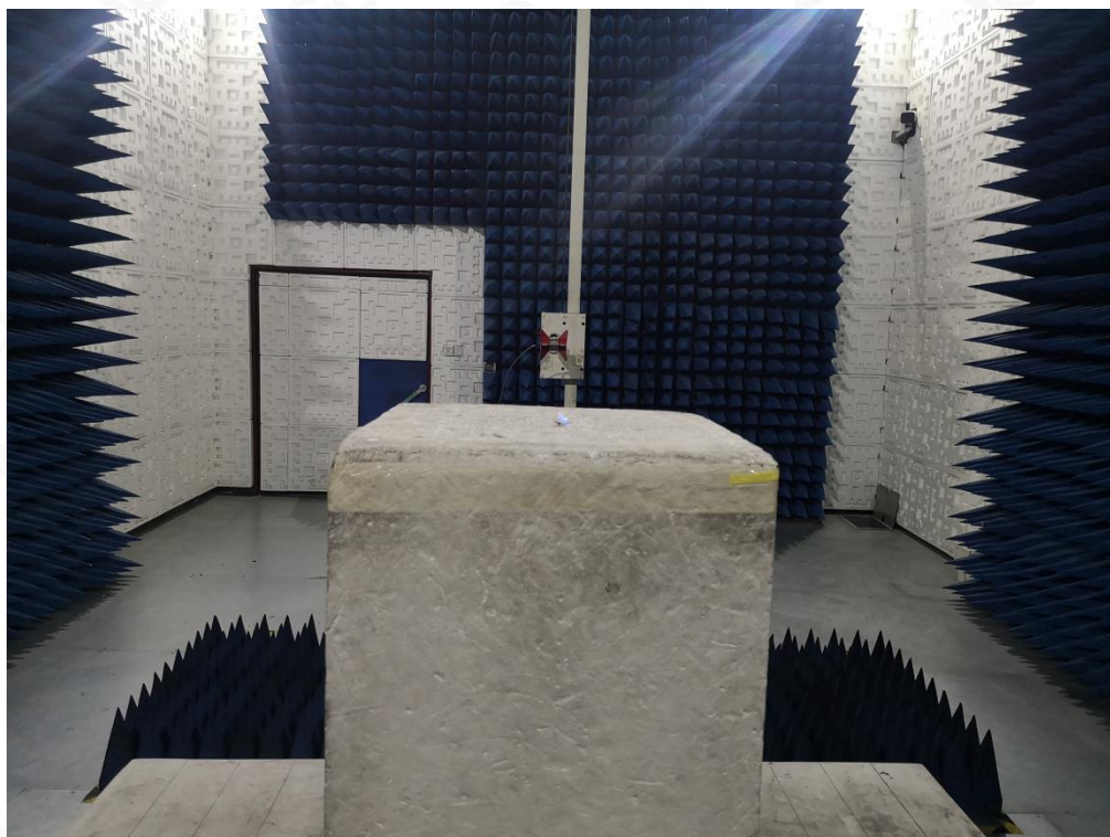
RADIATED EMISSION TEST SETUP ABOVE 1GHZ
