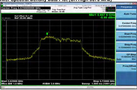
802.11n HT40, 5470~5725 MHz Peak Power Spectral Density Data Plot (CH High 5710 MHz)
