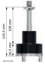
Measuring the antenna height - pillar setup
