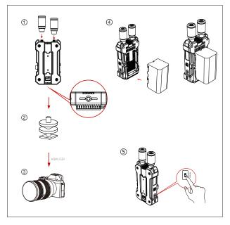
① Install the antenna shown in the picture.
