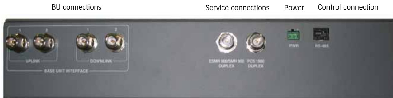
Figure 2. RIU Lite Rear Panel
