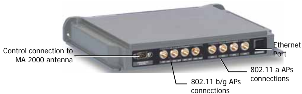
Figure 2-15. MobileAccess 850 Rear View
