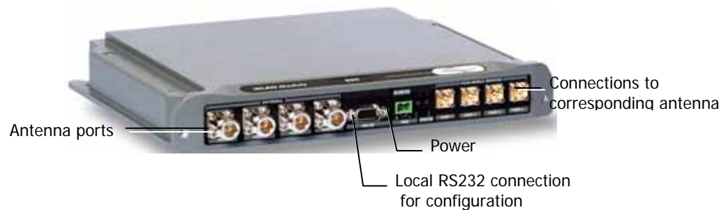
Figure 2-14. MobileAccess 850 Front View
