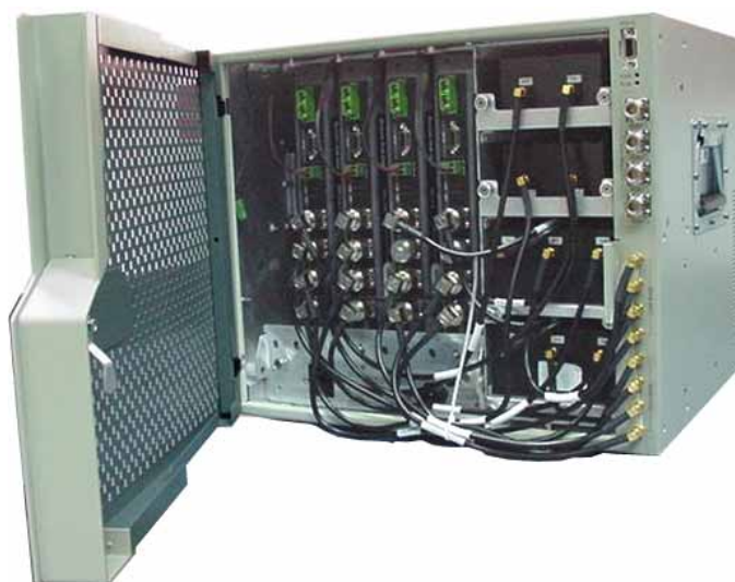
Figure 2-18. RC Open Cabinet with Internal Cabling
