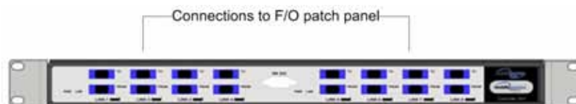
Figure 4-3. BU Front Panel Connections
