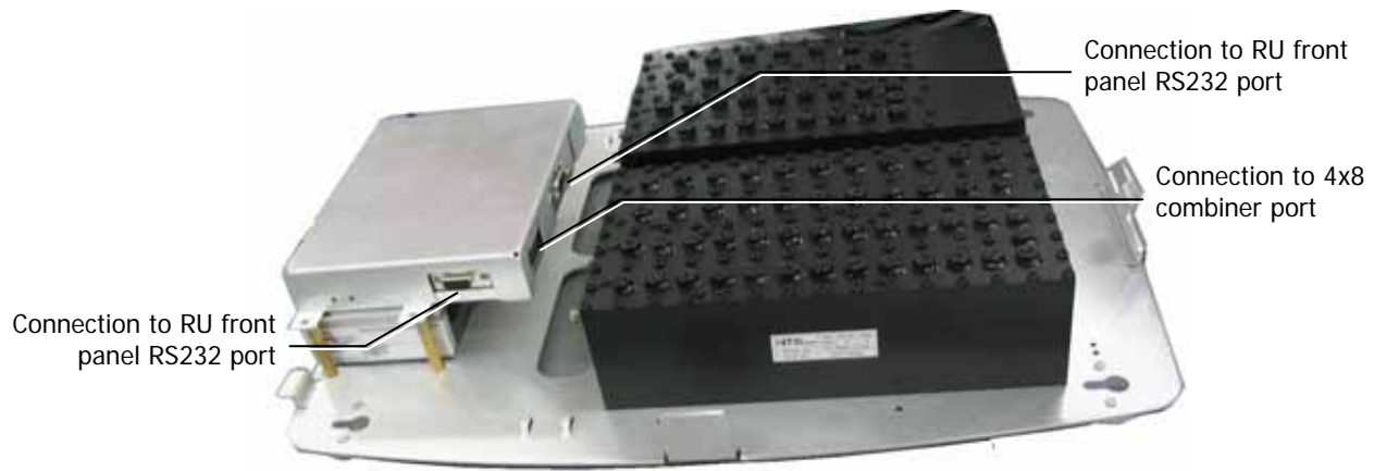
Figure 4-13. Side View of the Open MA 2000 without the Cables
