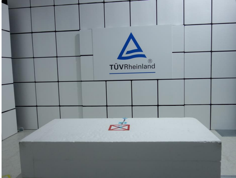
Photograph 2: Test Setup for Spurious Emissions (Front View 2)
