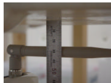
Fig. 21. Body SAR Test Setup with Holster
