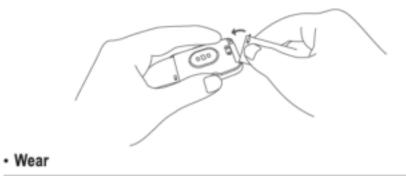
Wear the device to a finger-wide distance from the wrist bone, and adjust the tightness of the wrist strap to a comfortable position. In order to get a best measurement results, the back of the device needs to be in contact with the skin.
