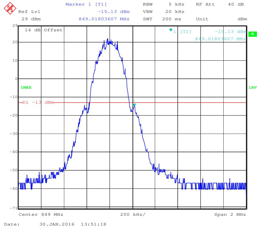
**PCS Band, Left Band Edge for GSM (GMSK) Mode**
