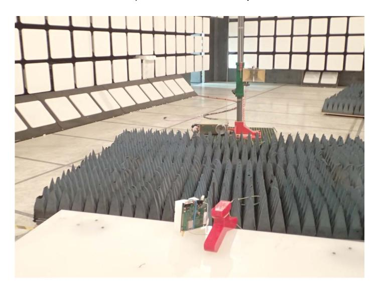
${\bf Radiated\ Emissions\ @\ 3\ m} \\ {\bf EUT\ with\ 3.3\ dBi\ Monopole\ (Integrated\ Whip)\ Antenna\ and\ 0.44\ dB\ Assembly\ Cable\ Loss}$
