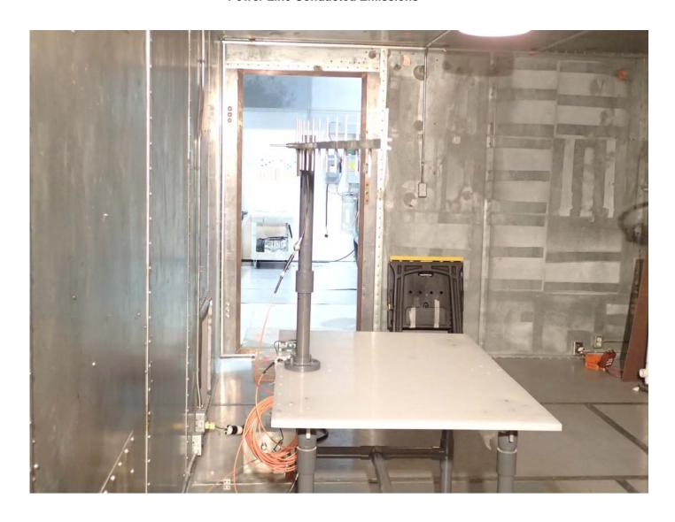
Radiated Emissions @ 3 m, Orthogonal Position 1 EUT with 8.1 dBi Omni-directional Antenna and 2.85 dB Assembly Cable Loss
