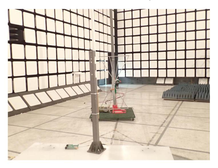
Radiated Emissions @ 3 m, Orthogonal Position 2 EUT with 14.0 dBi Yagi Antenna and 9.86 dB Assembly Cable Loss
