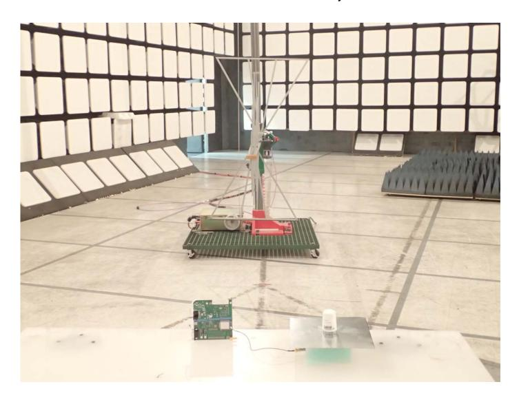
Radiated Emissions @ 3 m EUT with 2.1 dBi Dipole Antenna and 0.36 dB Assembly Cable Loss
