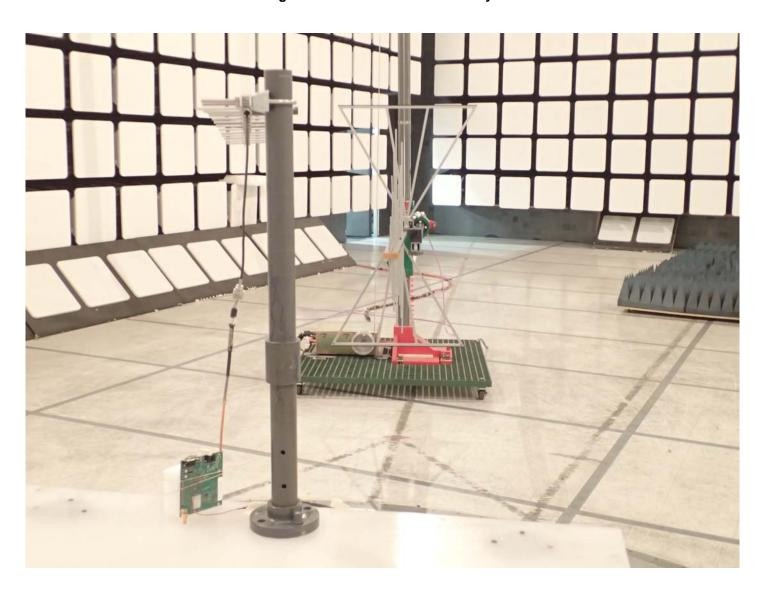
Radiated Emissions @ 3 m, Orthogonal Position 3 EUT with 3.0 dBi Dome Antenna and 0.44 dB Assembly Cable Loss
