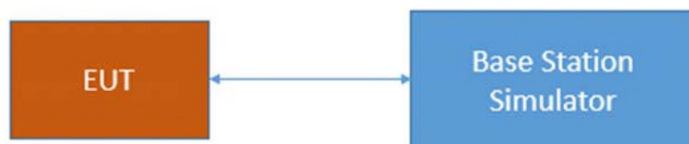
Test Setup FCC Part 22/24/27/90 Cellular; Frequency stability
