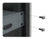
Fig.5 Fix AU with Screws
