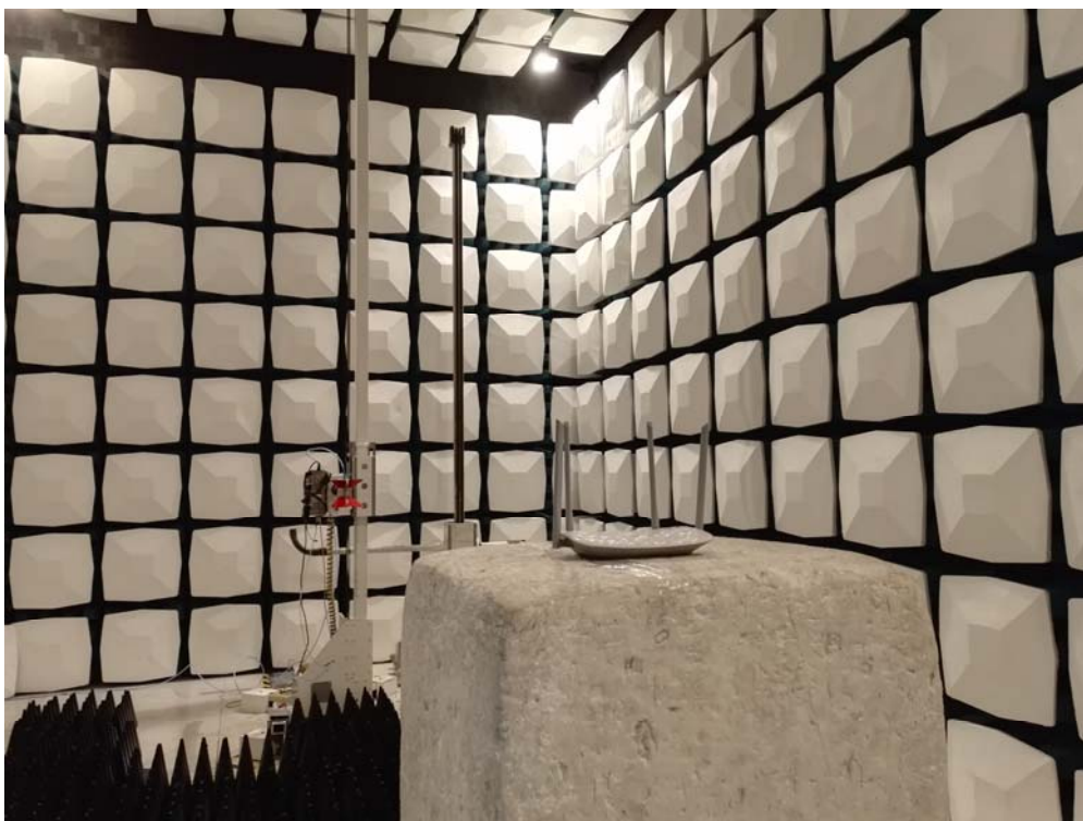
Description: Radiated Emission Test Setup for 1~18GHz
